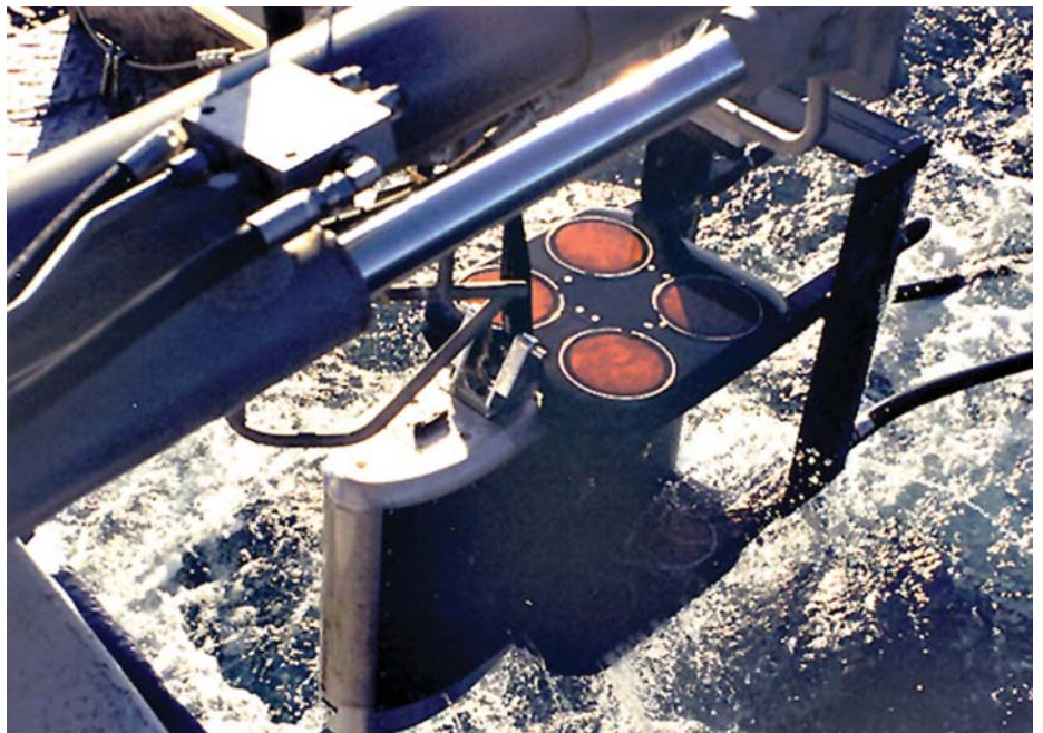
The low frequency designed into the LFATS using proprietary transducer and beam-forming technology allows multiple boundary interactions and reduced reverberation contamination of the received signals.
