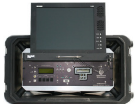
The Generation IV GCS control panel with pull-out payload monitor extended; front view.
