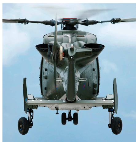
This rear view shows the distinctive exhausts fitted to the Wildcat. (Photo: AgustaWestland)
