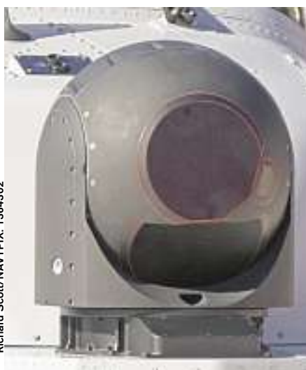
■ The L-3 Wescam MX-15Di electro-optical/laser designator system – combining IR, TV and laser designator subsystems in a nose-mounted turret – will meet the needs of the UK's battlefield and maritime variants.
