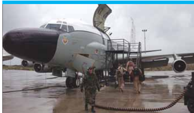
An RC-135 Rivet Joint aircraft ready for a mission. This electronic surveillance aircraft has seen extensive use in Afghanistan. (US Air Force)
