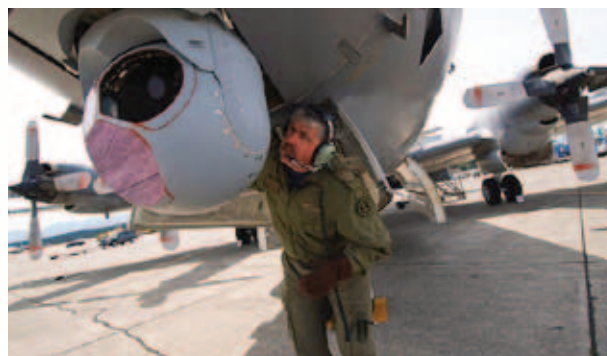
L-3 WESCAM supplies EO/IR equipment for the CP 140 Aurora
