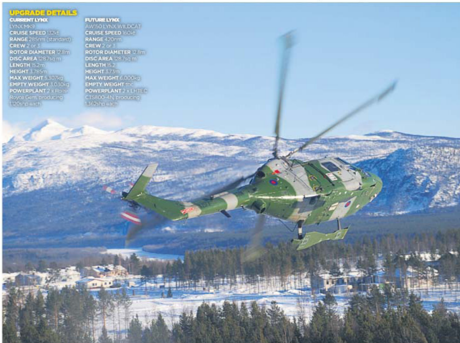
* Recently revised semi-rigid four-blade rotor assembly will be retained, vital for carrier-borne use.
