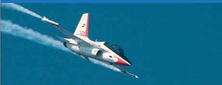
Clearly showing its F-16 heritage, the Mach 1.4 Korea Aerospace Industries-Lockheed Martin T-50 Golden Eagle is the only supersonic advanced trainer currently in large series production. (Armada/EHB)
