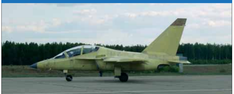
Providing a major advancement in thrust/weight ratio and usable angle of attack, the Yakovlev Yak-130 is shown here in the form of the first production aircraft for the Russian Air Force, built by Sokol. It was photographed ten days after its maiden flight in May 2009. (Yakovlev)
